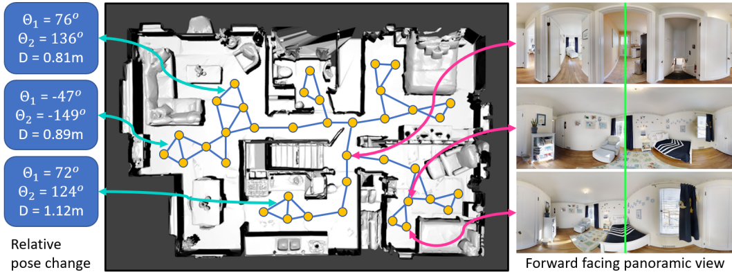
Figure 1: An illustration of the learned panoramic topological memory (PTM) after exploring the environment. Each vertex is a recorded panoramic view observation with center to be the front face direction of the agent. Each edge records the relative pose difference required to travel from one to another via local controller.
